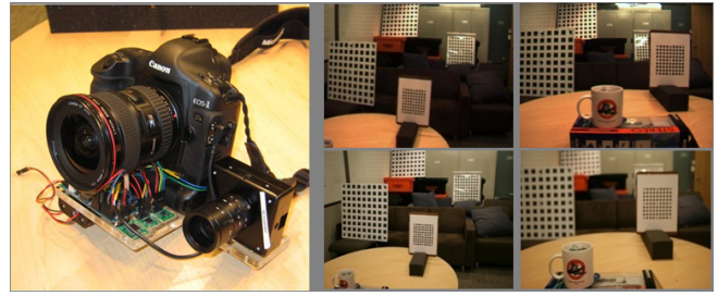
Figure 4: Ground Truth Blur Measurements: We attach a high-speed camera next to an SLR and capture high-speed video frames during the camera exposure. With additional wide-baseline shots, we perform 3D reconstruction using bundle adjustment. We show our high-speed camera attachment and a few images from the high-speed camera (we took about a hundred total for the process).
